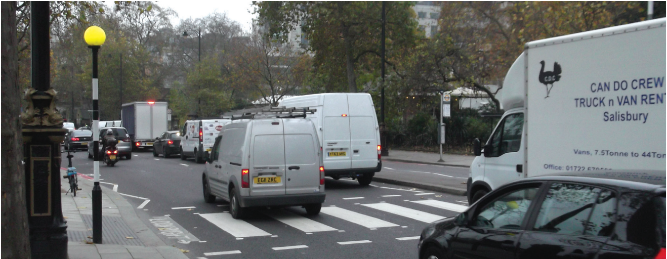
Multi-lane approaches to crossings can create issues where pedestrians are “masked” by slow moving or stationary traffic
