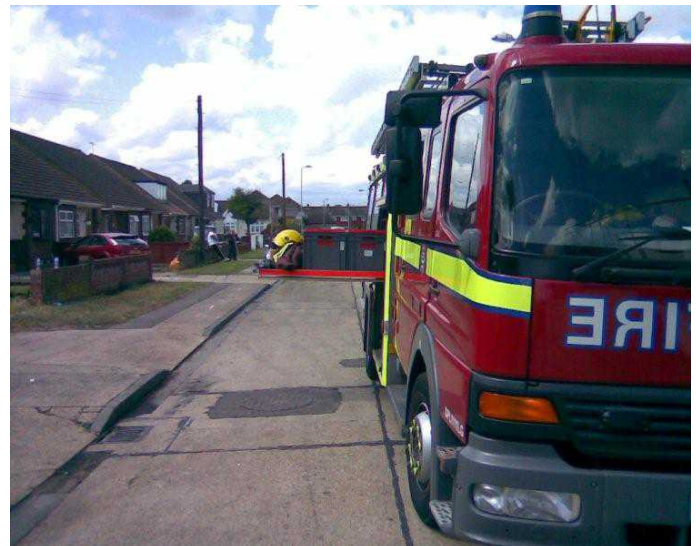
Fire appliance (London Fire Brigade) showing equipment access from the side of the vehicle.
