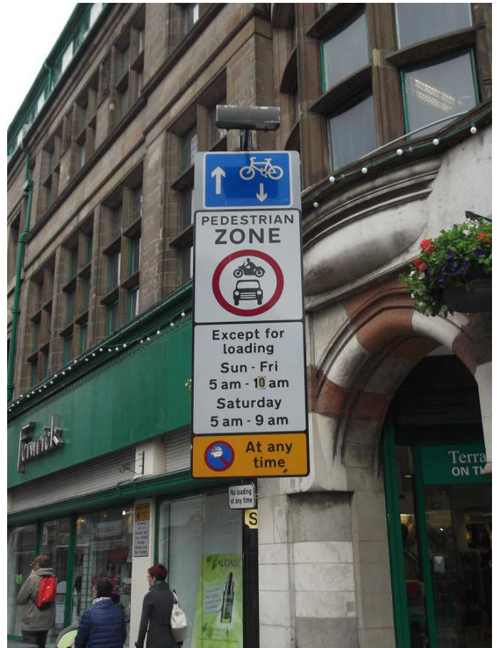
A pedestrian zone with the "no motor vehicles" sign actually permits cycling. Here, two-way for cycling, one-way for motors.
