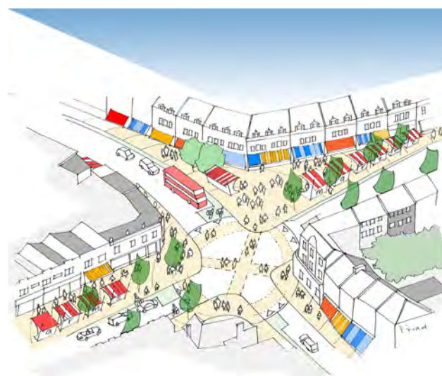
Diagonal pedestrian crossing reflect desire lines
