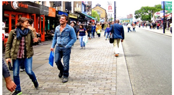
Raised level loading/parking bays Camden High Street. Vans unload here early morning, rest of the time available for people/customers.
